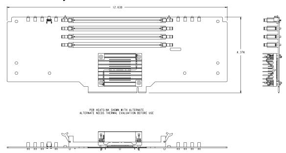
Figure 21. Memory Board Mechanical Outline Drawing
